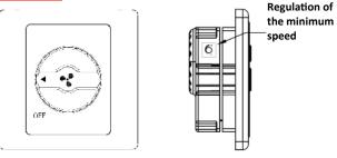
1. Fan speed can be adjusted by rotating the knob:
