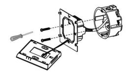
3. Connect the LCD board into the wall plate.
