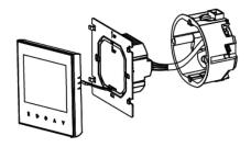
2. Fix the wall plate into the wall box by a screwdriver.
