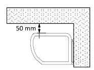
The width of the curtain should be greater or equal to the width of the door frame.
