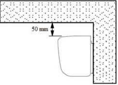
The width of the curtain should be greater or equal to the width of the door frame. When the entrance is wider than the unit, it is recommended to install two or more units in parallel. In this case, provide 10-40 mm gaps between the units.
