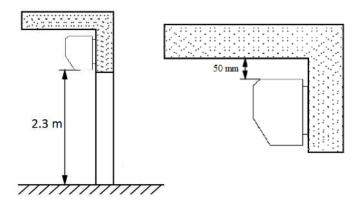
The width of the curtain should be greater or equal to the width of the door frame. When the entrance is wider than the unit, it is recommended to install two or more units in parallel. In this case, provide 10-40 mm gaps between the units.
