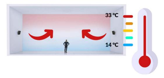
Temperature distribution **WITH** the use of **DESTRATIFICATON FAN.**
