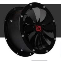
The destratification fans circulate warm air from the ceiling area to the human occupied zone. So in a sense, they limit an undesirable phenomena of vertical temperature gradient. This way of using the device allows for effective utilisation of the supplied air, providing thermal comfort of people staying in the building.
